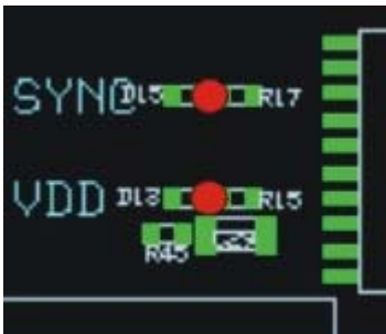
LED's for Module active power and network connection
