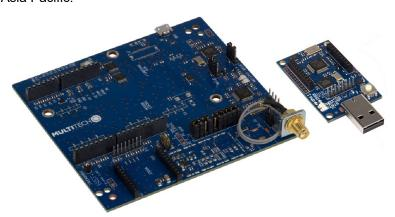
For developing with the mDot, the Starter includes both the mDot Micro Developer Kit and the full-sized mDot Developer Kit. Both options allow you to plug in the mDot and use it for testing, programming, and evaluation. The portable design of the Micro Developer Kit makes it ideal for connecting to a laptop and doing LoRa network doing range testing.
