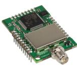
The mDot is a secure, Arm<sup>®</sup> Mbed<sup>TM</sup> programmable, low-power RF module that provides long-range, low bit rate M2M data connectivity to sensors, industrial equipment and remote appliances. LoRaWAN certified, the mDot provides bi-directional data communication up to 10 miles/15 km line-of-sight and 1-3 miles/2 km
