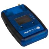
The mDot™ Box helps you determine if LoRa® is the right technology to effectively connect to and manage thousands of assets and sensors in the field to while meeting your company's cost, performance, and strategic needs. The mDot Box pairs an mDot RF module with built in sensors including temperature, ambient light, pressure, electrical current. and a 3-Axis
