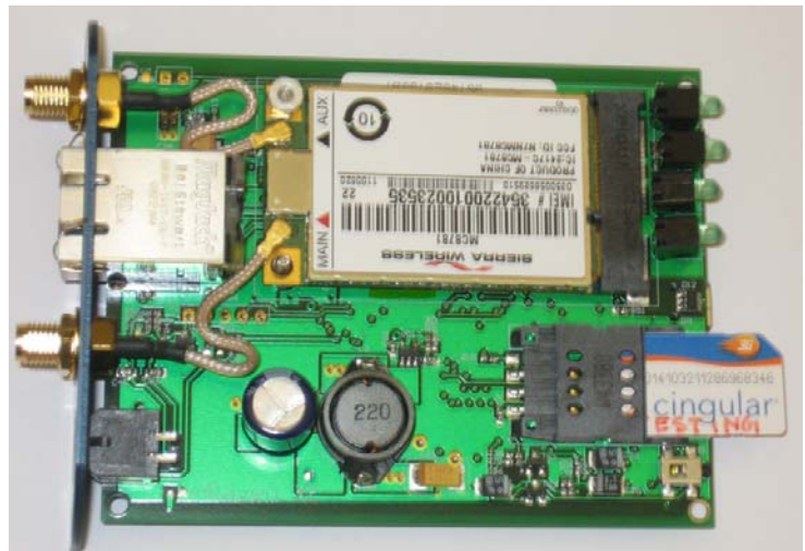
Figure 0-3: Insert SIM in to the modem
